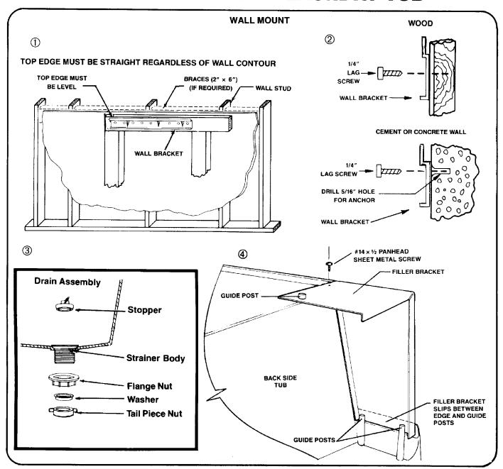
① Break off left side of wall bracket by snapping along the bracket's scored ridge.
