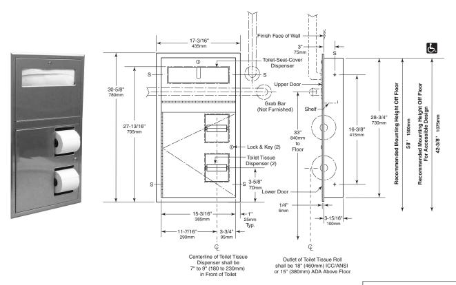
Rough Wall Opening 16" (405mm) wide 29-1/4" (745mm) high 4" (102mm) minimum recessed depth
