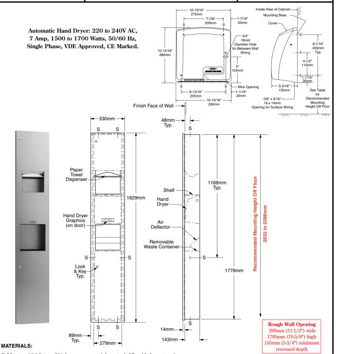
$\textbf{Cabinet} \ -- \ 18\text{-}8 \ S, \ type-304, \ heavy-gauge \ stainless \ steel. \ All-welded \ construction.$
