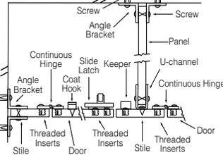
Standard gaps are provided at all walls and between components to allow for hardware attachment. Wall gaps are standard 1/2" to 1"
